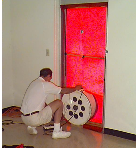
Picture 26. Back side of a blower door apparatus.
