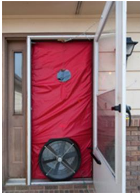
Picture 25. Front side of a blower door apparatus.
